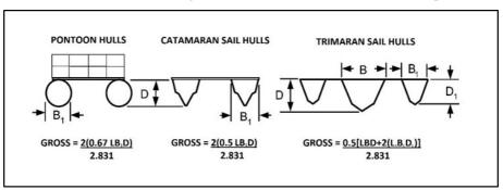
Where L is the length of the centre hull and  $L_1$  is the length of the outside hulls.
