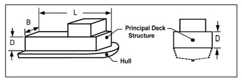
(2) For the purpose of sub-paragraph (1), a deck structure is considered excessive in size if the tonnage of the principal deck structure calculated using the following formula is equal to or exceeds the total gross tonnage of all of the pleasure craft's hulls:
