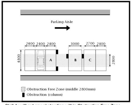
Stall A: without any obstruction within Obstruction Free Zone Stall B: with obstruction on both sides Stall C: with obstruction on one side
