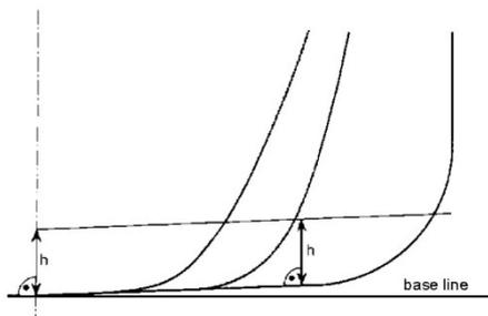
**Figure 1 — Oil fuel tank boundary lines
