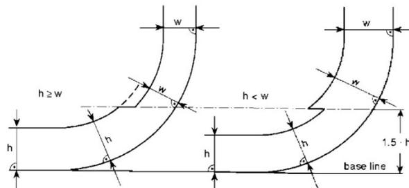
**Figure 2 — Oil fuel tank boundary lines
