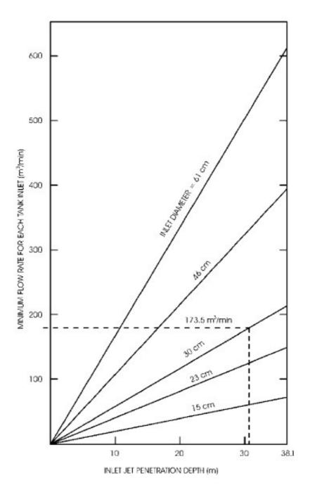
Figure 7–1. Minimum flow rate as a function of jet penetration depth.
