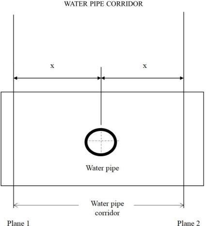
1.--(1) Where "X" is the distance of each of Plane 1 and Plane 2 from the centreline of the water pipe and is ----
