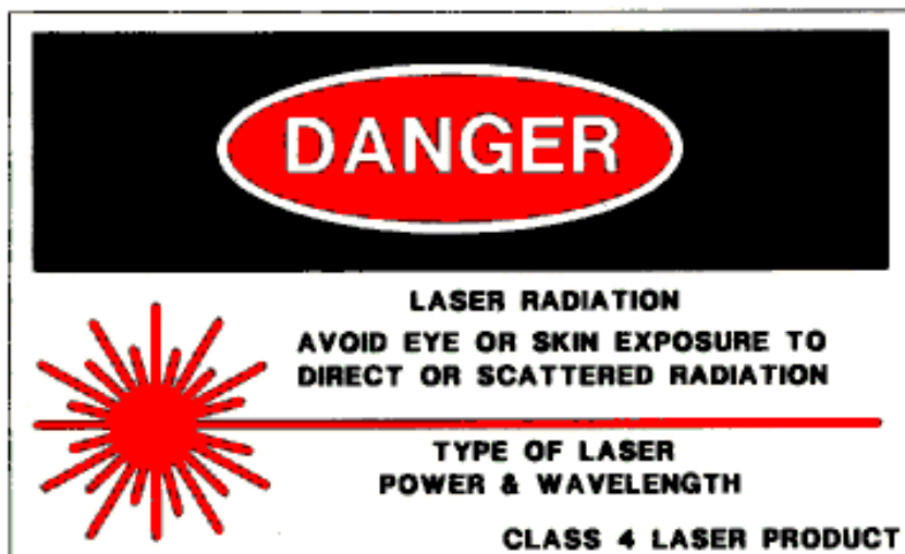
FIGURE 4 Warning Label for Class 4 Laser Product
