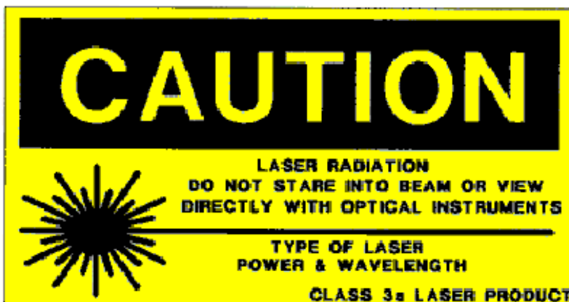
FIGURE 2 Warning Label for Class 3a Laser Product
