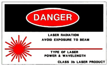
FIGURE 3 Warning Label for Class 3b Laser Product
