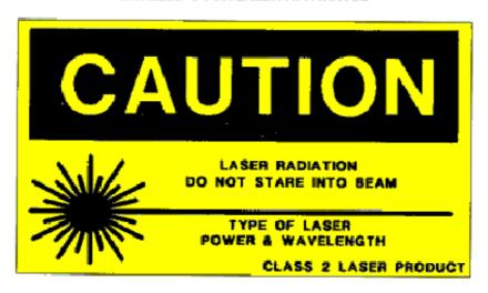
FIGURE 1 Warning Label for Class 2 Laser Product
