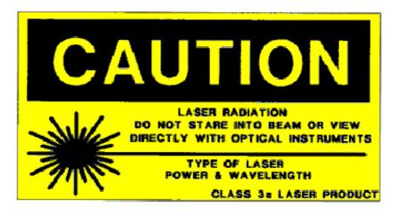
FIGURE 2 Warning Label for Class 3a Laser Product
