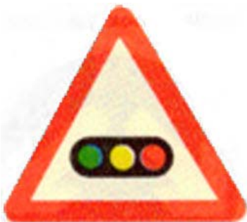
TRAFFIC SIGNALS AHEAD
