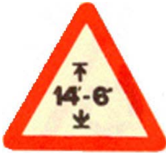
HEIGHT LIMIT E.G. LOW BRIDGE
