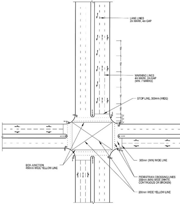
MARKINGS INDICATING A PEDESTRIAN CROSSING AT A SIGNAL-CONTROLLED JUNCTION
