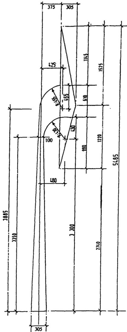
This marking indicates that vehicles on the lane with the marking may only turn right.
