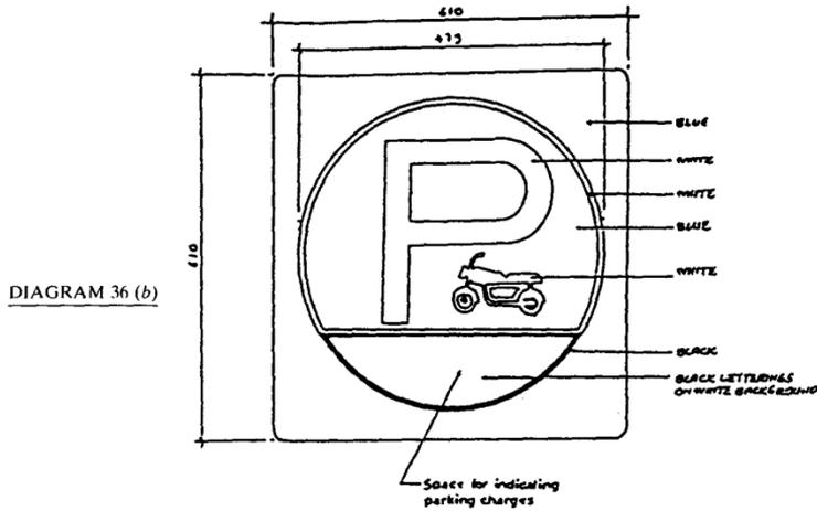
This sign indicates a designated pay parking place for motor vehicles with less than 4 wheels and the weight of which unladen does not exceed 470 kilograms.
