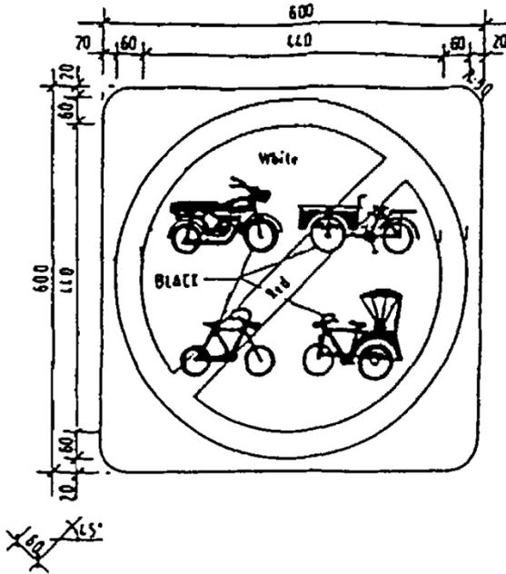
MOTOR CYCLES, POWER-ASSISTED BICYCLES AND PEDAL-CYCLES RESTRICTION
