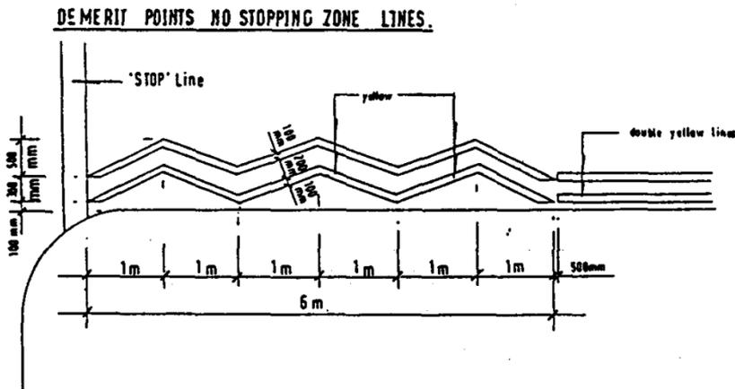
Double zig zag yellow lines at the edge of a road prohibiting stopping of vehicles at all times unless the vehicle is prevented from proceeding due to traffic conditions.
