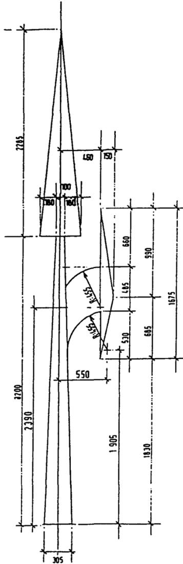
This marking indicates that vehicles on the lane with the marking may only proceed straight ahead or turn right.
