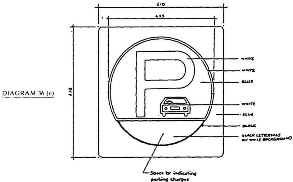
This sign indicates a designated pay parking place for motor vehicles, the weight of which unladen does not exceed 1,500 kilograms.
