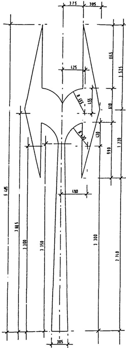
This marking indicates that vehicles on the lane with the marking may only turn left or right.
