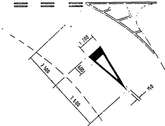
Marking indicating that vehicles are required to give way to traffic on the right or left, as the case may be.
