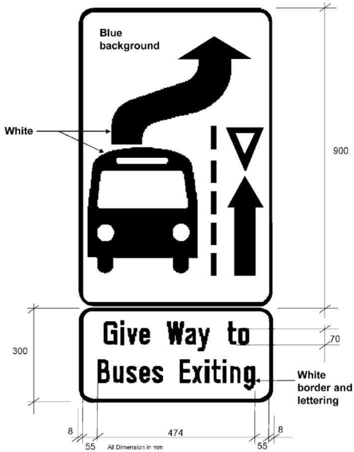
This sign indicates that vehicles shall stop before the Bus Give-Way Line and give precedence to any bus entering or waiting to enter the Bus Give-Way Box.
