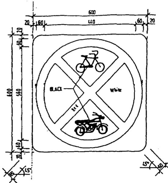
This sign prohibits the parking of motor vehicles with less than 4 wheels weighing not more than 470 kilograms.
