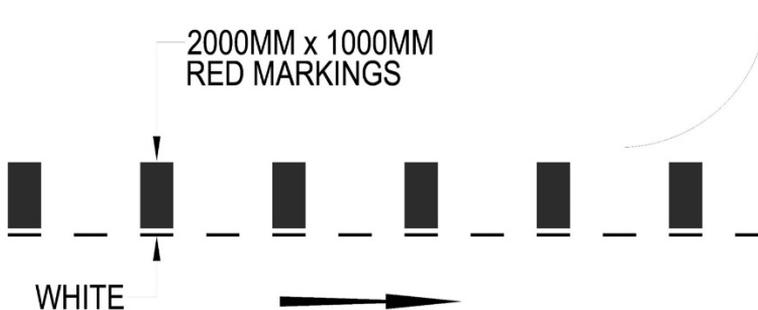
The red transverse lines of not less than 1,000 mm in width are laid down perpendicular to the edge of a road. These lines indicate that the parking of any vehicle is prohibited along the length of the road starting from the point where those lines are indicated, to the point the lines end.
