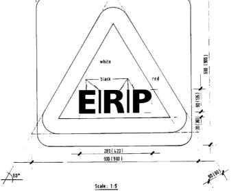
Note: Dimensions in brackets are for signs installed on expressway
