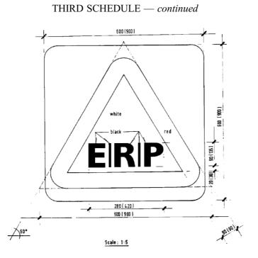
Note: Dimensions in brackets are for signs installed on expressway
