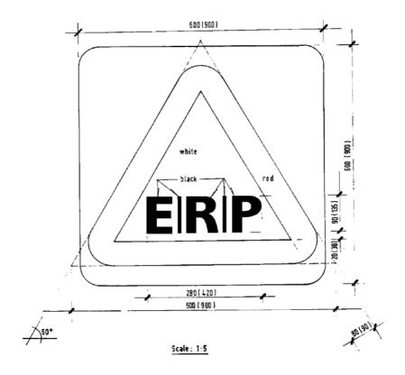
Note: Dimensions in brackets are for signs installed on expressway
