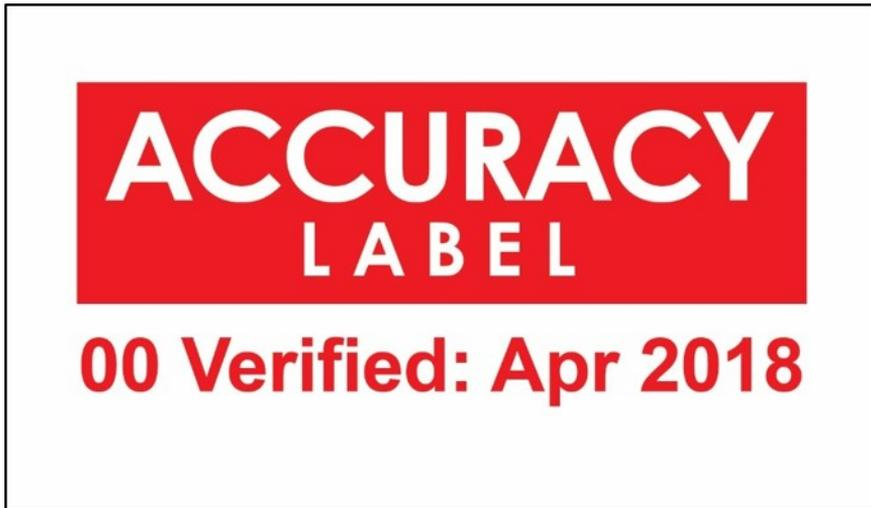
where “Apr 2018” (as shown in the illustration above) represents the month and year in which the weighing or measuring instrument is passed as fit for use for trade.
